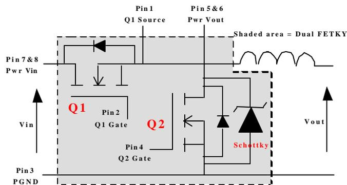
Pin nomenclature has been changed to represent a functional block in order to make it easier to interface with the rest of the system. Conventional discrete component terminology is removed to be replaced with more conventional power conversion terminology, like PGND, Pwr Vin, Pwr Vout, etc. The Dual FETKY specification is shown in Table 1.
