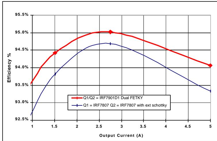
For 5.0V applications, up to 1% advantage across all load conditions can be obtained
