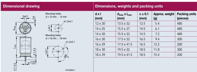
The PC board hole arrangement specified above is based on circular arcs.
