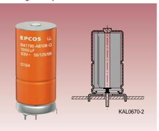
1 mm wires and corrugation for increased vibration stability, enhanced further by soldering star design.
